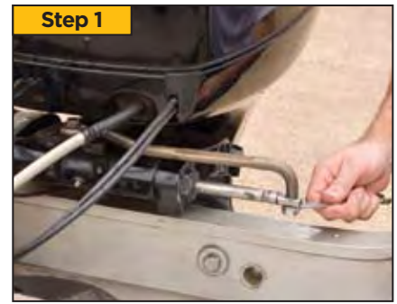
The Steersman Steering Guard replaces the factory nut on the port side of the outboard tilt tube. The steering rod, which is part of the cable assembly, passes through this nut as the boat is steered.
